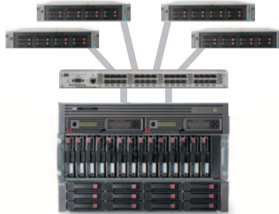
MSA1500 attached to an MSA20 and MSA30 and connected to four HP ProLiant DL380 servers via a Fibre Channel switch attached to the 2U controller shelf with Selective Storage Presentation
