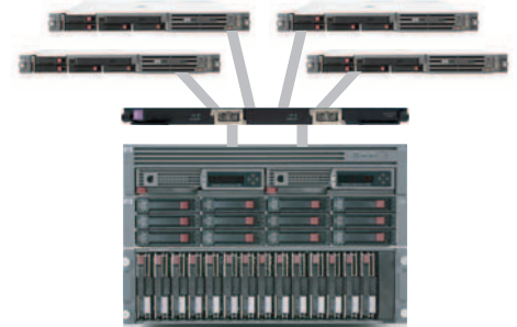
MSA1510i with MSA30 and MSA20 enclosures, connected via a Procurve Gigabit Ethernet Switch to four ProLiant DL360 servers
