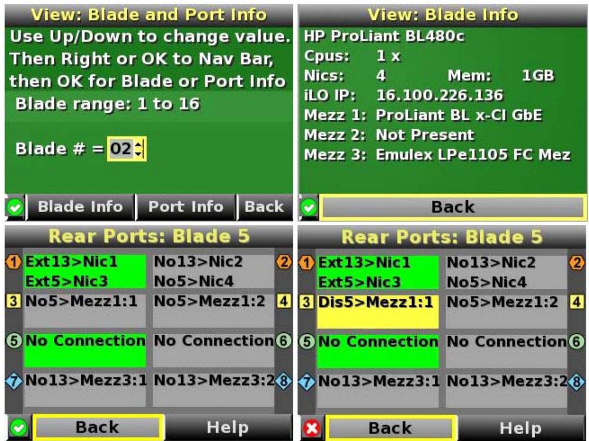
Figure 8. Illustration depicting the Blade and Port information screens; Blade and Port selector screen (top left), Blade Info screen (top right), Rear Port summary screen indicating no errors (bottom left), Rear Port summary screen indicating errors (bottom right).
