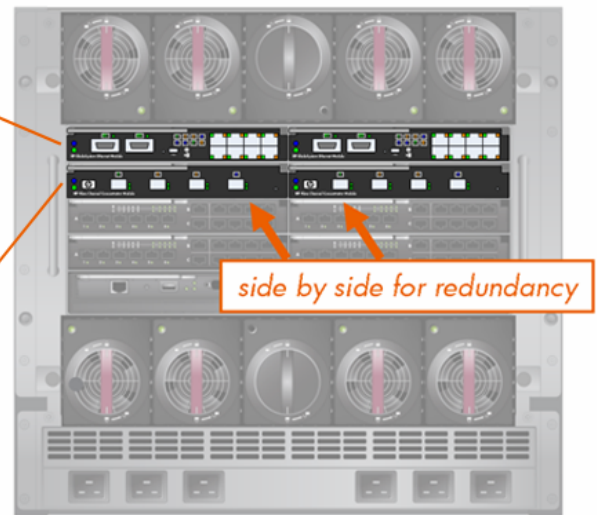
Figure 3. Illustration depicting the Virtual Connect modules in the HP BladeSystem c7000 enclosure
